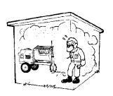
any enclosed or narrow area where free flow of the air is restricted. If the air flow is restricted it will cause serious damage to the mixer or engine and may cause injury to people. Remember the mixer's engine gives off DEADLY carbon monoxide gas.
